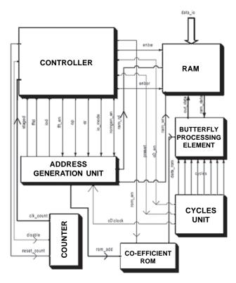
Figure 2: The FFT Processor
