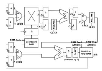
Figure 3: Butterfly Processing Element
